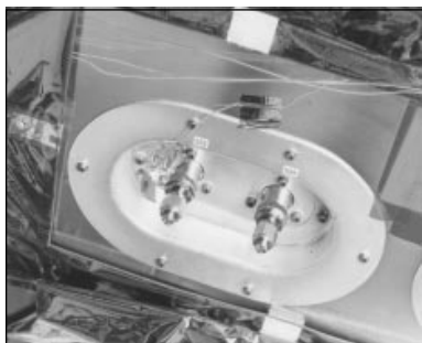
Fill and Drain Valve
