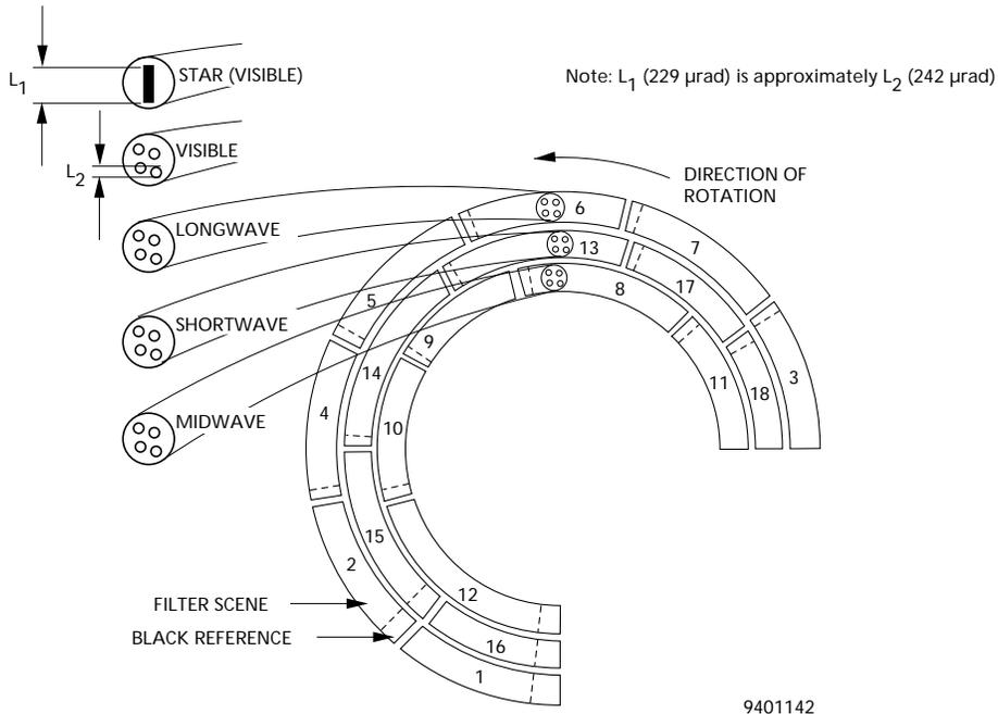
period for maximum stability and coregistration. Though not viewed through the filter wheel, the visible detectors are gated so that they sample the same atmospheric column at the same time as the IR channels.
