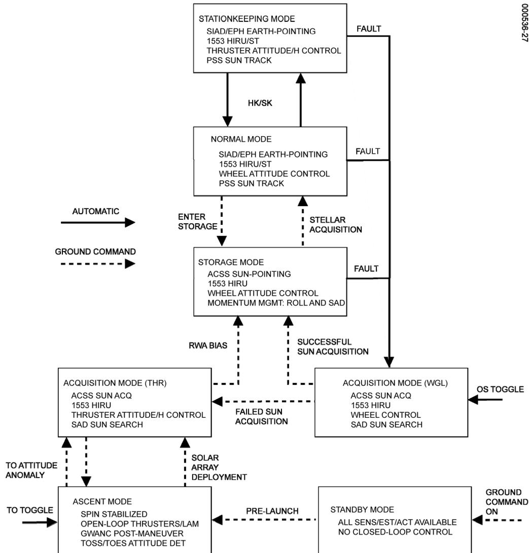
**Figure 11-2. GOES Attitude Control Electronics Operational Modes**
