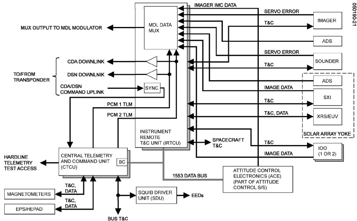
**Figure 9-2. Telemetry and Command Digital Subsystem Configuration (Half-diagram)**
