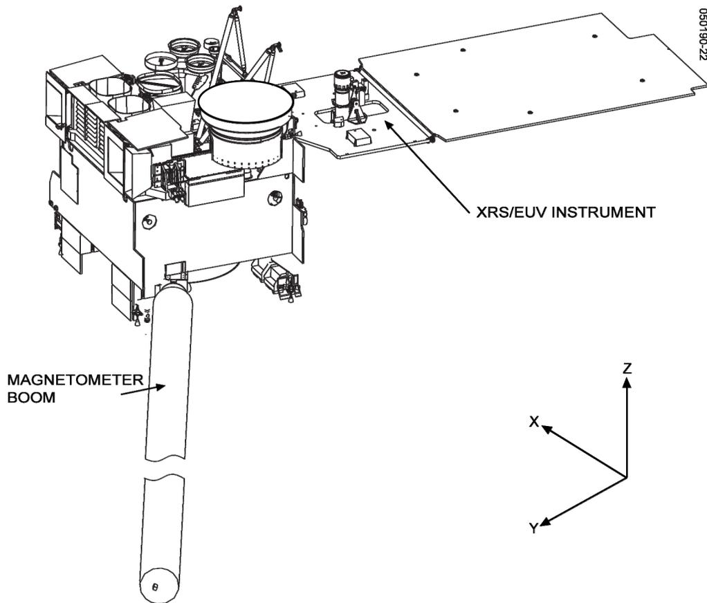
**Figure 5-2. Deployed XRS/EUV Instrument – Schematic View**
