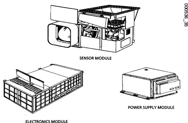
**Figure 3-2. Imager Instrument Modules**
