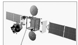
Original architecture of Elektro-L satellite circa 2001. Credit: NPO Lavochkin
