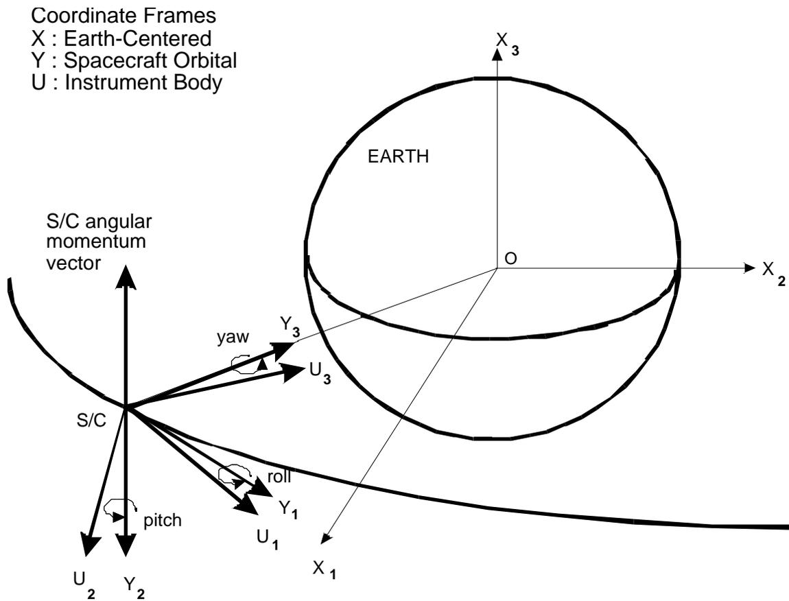
**Figure 4-1. Spacecraft Coordinate System Geometry**
