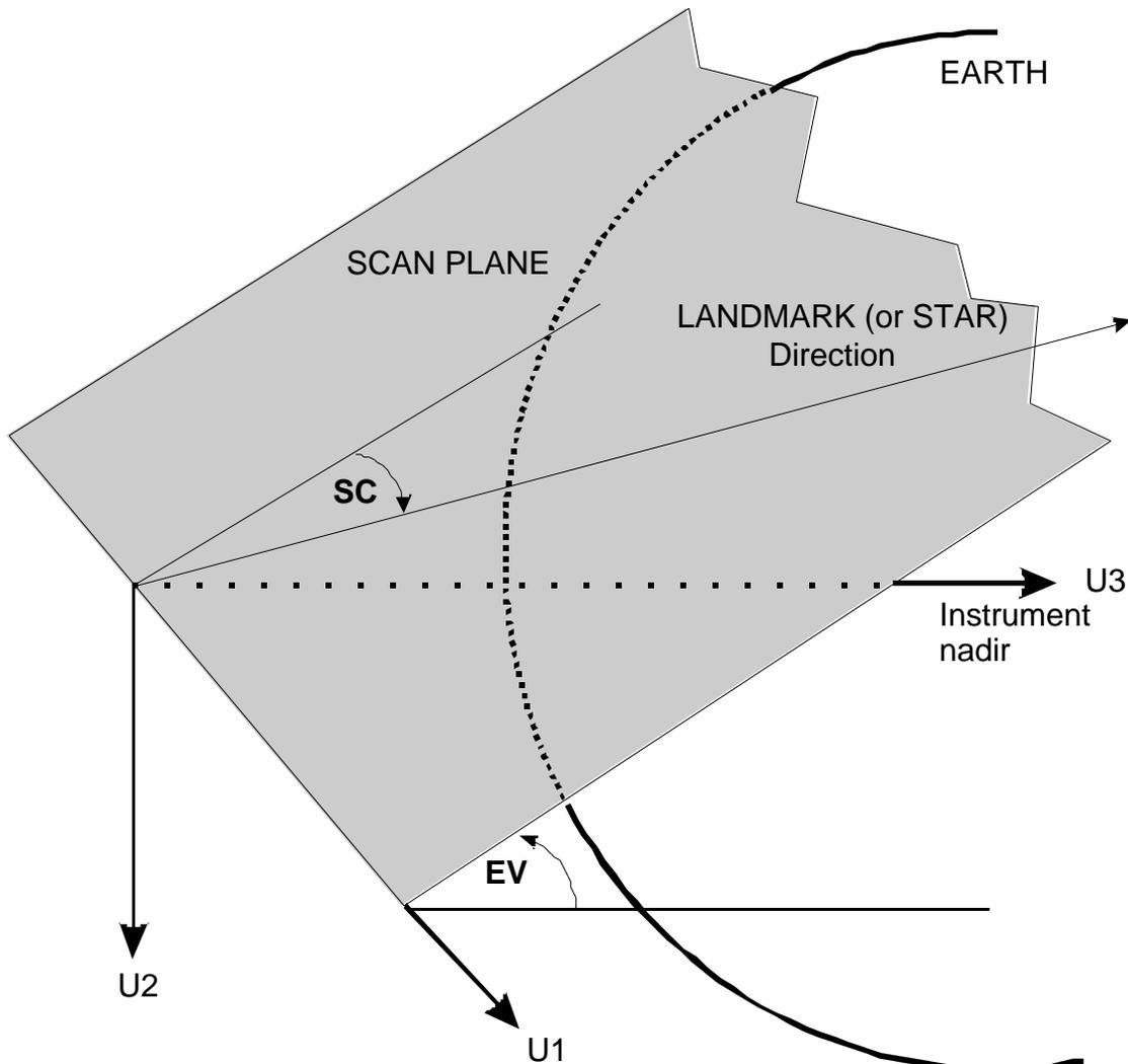
**Figure 4-2. Instrument Angle Geometry**
