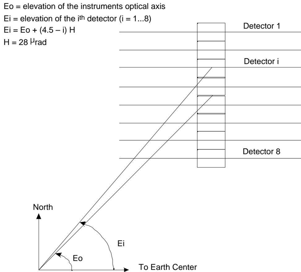
**Figure 3-5. Instrument Optical Axis and Detector Pointings**
