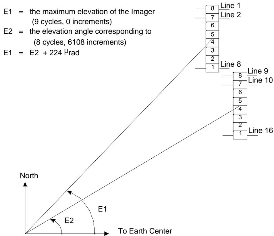
**Figure 3-4. Elevation and Line Coordinates of the Imager for a Flipped Spacecraft**
