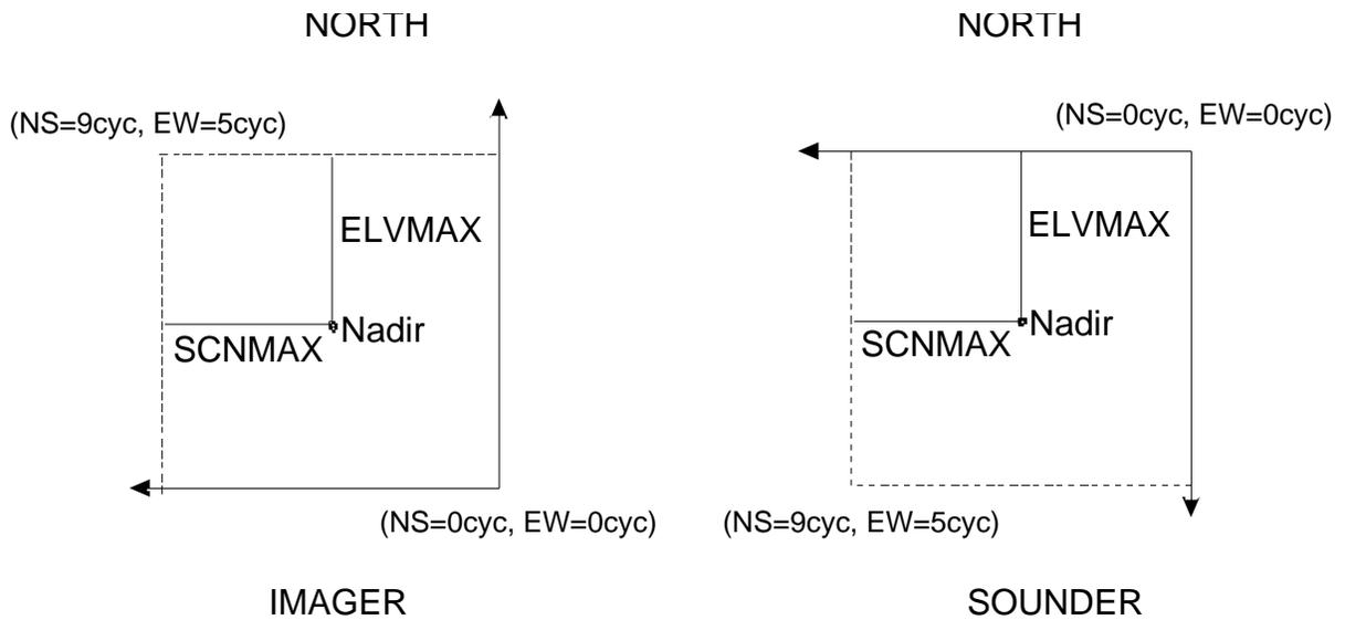
**Figure 3-2. ELVMAX and SCNMAX for a Flipped Spacecraft**
