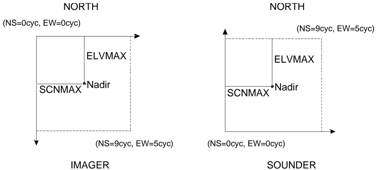
**Figure 3-1. ELVMAX and SCNMAX for a Normal Spacecraft**
