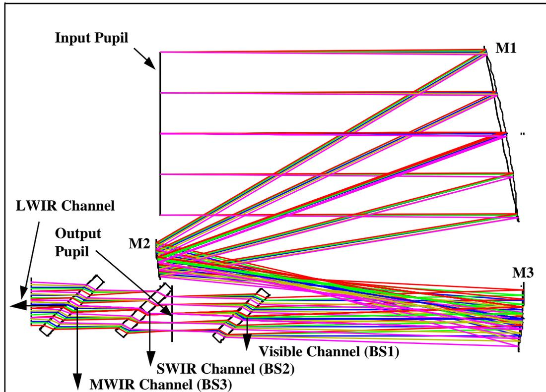
**FIGURE 3. Cassegrain Afocal Telescope Feeding Four Focal Plane Assemblies**
