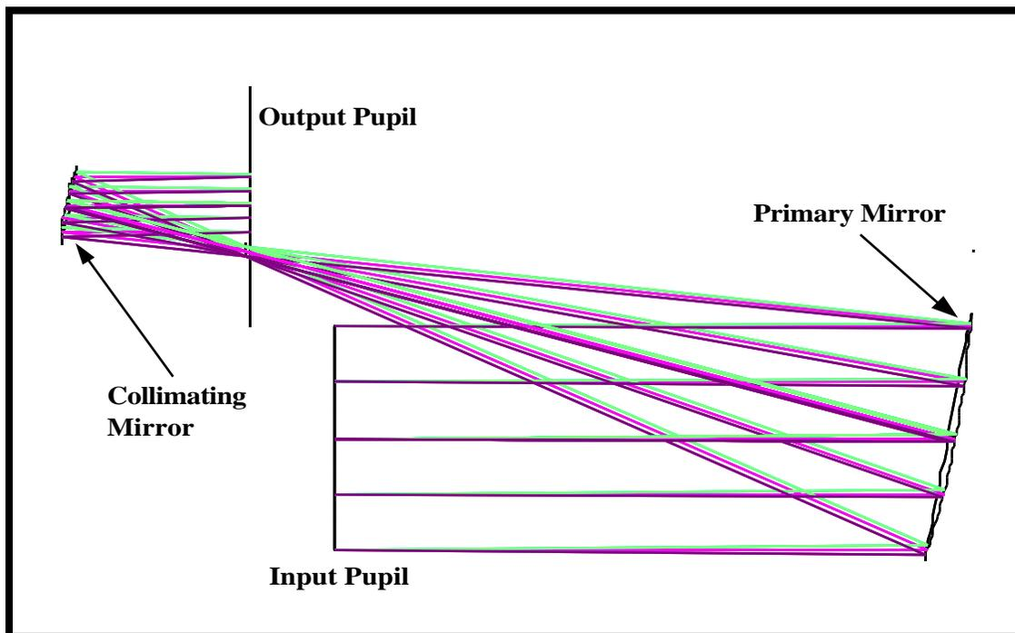
**FIGURE 2. The AGS Confocal Parabola 30cm Telescope. Curvature of field dominates**
