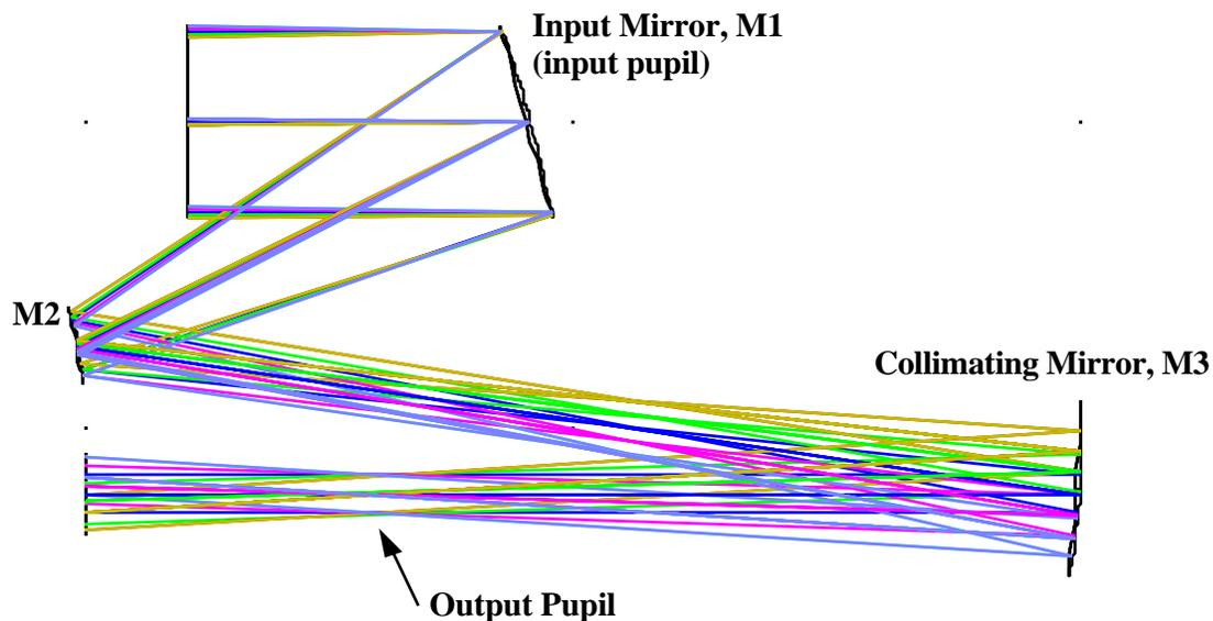
**Figure 1. Wide - Field 1.8 degree FOV 4.48X Afocal Anastigmat. M1 is 30cm diameter.**
